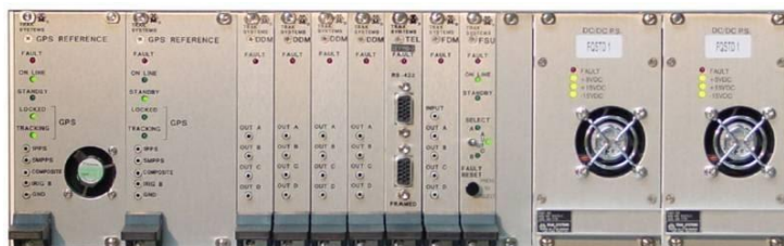
Figure 1-3: TRAK 9100 Simulcast Site Reference – Provides the simulcast system 1 PPS, 5 MPPS, and 1 PPS + 5 MPPS composite signals to synchronize the simulcast transmissions.
